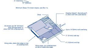
Apply as shown. Note: GAF-Elk Weather Blocker\* starter strips shingles are recommended at the eaves and rakes for best performance and required for the best limited wind warranties on certain products (see limited warranty for details).
