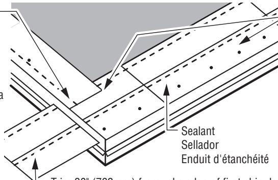
Place starter strip shingles 1/4" – 3/4" (6 – 19mm) over eave and rake edges to provide drip edge. Nail approximately 1-1/2" – 3" (38 – 76mm) above the butt edge of the shingle.
