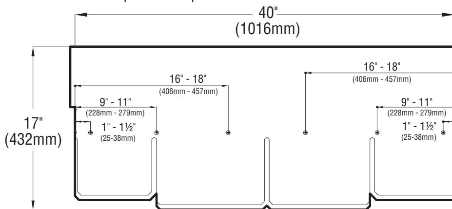
**ENHANCED NAILING PATTERN** - six nails per shingle\*
