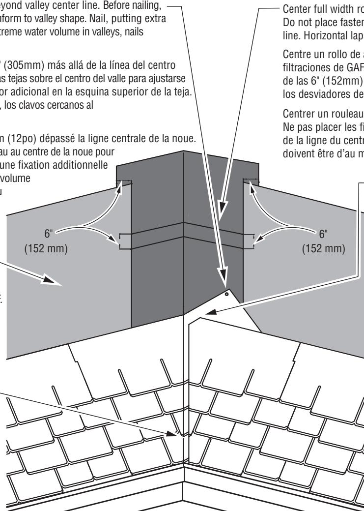
Center full width roll of GAF leak barrier. Do not place fasteners within 6" (152mm) of center line. Horizontal laps must be at least 6" (152mm).
